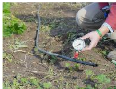
Figure 2: Measuring pressure using a pressure gauge at a lateral ending (Source: MREA, 2004).
